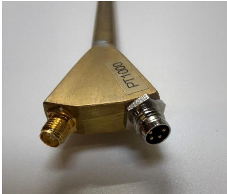
Sensor D = 30 mm L = 700 mm
